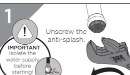
Clean and replace anti-splash as necessary. Secure in place
