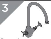
Turn on the mains water supply letting the water flow for a few minutes to flush through the system.
